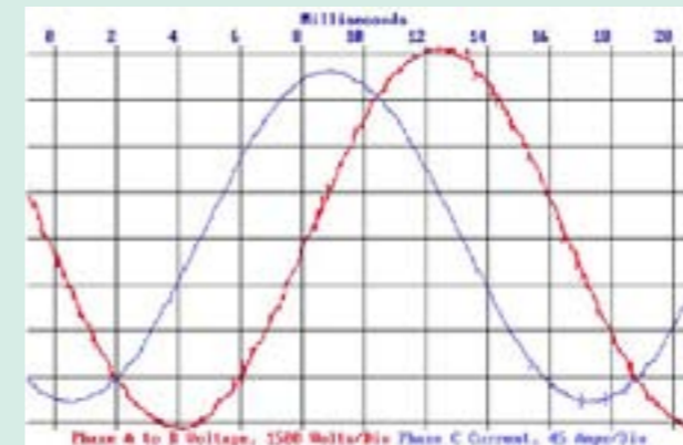
Figure 3 Power input without harmonic wave
